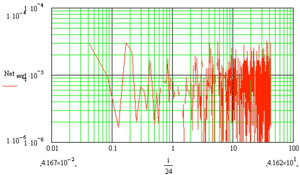
For the last graph above (#6), note the magnitude in the 0.1 Hz~0.02 Hz can be construed with noise where it may actually be small temperature shift or warm-up shift. I let the sensor stabilize for about 10 minutes before running the data but regardless, there is no temperature compensation done on the device.
