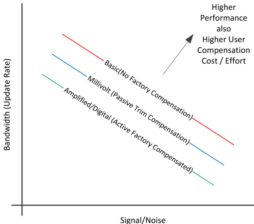
Figure 1: To get the highest performance for bandwidth and S/N, users may have to tradeoff an amplified version provided by the supplier and develop their own additional circuitry. Alternative pressure sensor products, such as All Sensors' Millivolt and Basic series (shown) provide an improved starting point.
